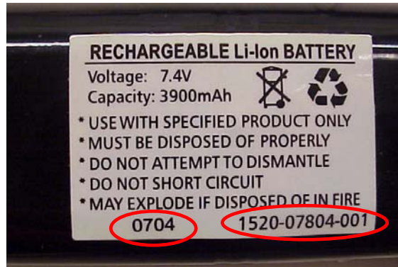
Battery Pack Date Code Example: 0704 (July 2004) Battery Pack Part Number Example: 1520-07804-001
